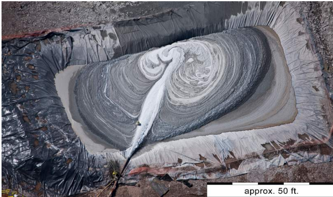
Figure 15. A waste pit in the Catskill Mountains containing drilling fluids from the hydraulic fracturing process. 41
